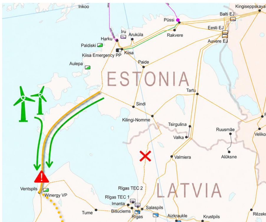
Figure 4: Illustrative N-1 contingency scenario showing the impact of high offshore wind generation from Kotlandi and additional power flows from mainland Estonia.
